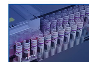
Sample Loading Module-Sample Scanning 350 sample positions, 450 samples delivered per hour
